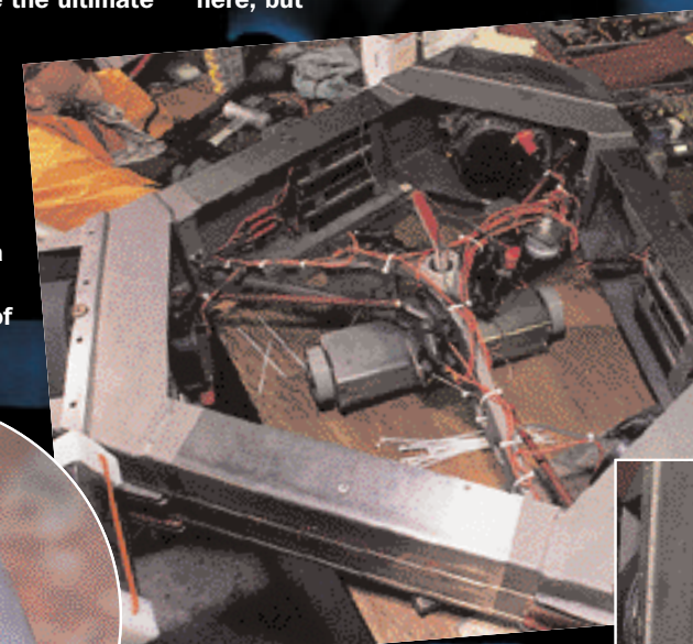
Y-Pout's frame (above) is made from welded titanium. The lid (removed) is steel.
